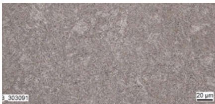
Tempered state, water cooled 200:1
